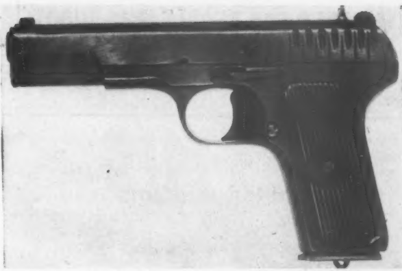
Tokarev 1930 pistol in 7.62 mm. caliber is short recoil operated Browning type with eight-round magazine. It measures 7 1/4 inches overall
